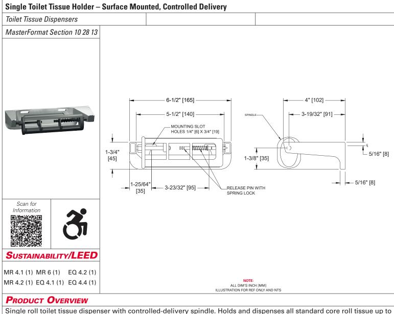
Single roll toilet tissue dispenser with controlled-delivery spindle. Holds and dispenses all standard core roll tissue up to 6" diameter [Ø152]. Fabricated of heavy-duty aluminum casting with satin-matte, silver-grey powder coated finish.
