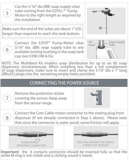
NOTICE: If the 4 contacts connectors are not connected properly, the motor will run continuously.
