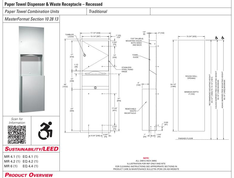
Dispenses 600 C-fold or 800 multi-fold paper towels. 12 gal. (46 L) stainless steel waste receptacle. Towels are self-feeding until supply is depleted. Unit may be reloaded with a partial load in-place and will continue to feed properly. Waste container is emptied manually on cycle determined by maintenance needs. Locking compartment and receptacle retainer prevents unauthorized access or removal.
