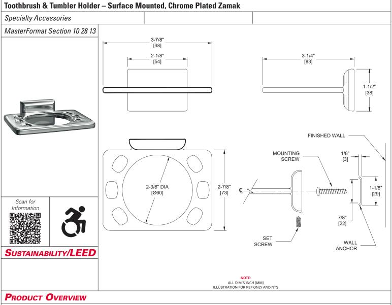
Fabricated from triple chrome-plated rust resistant Zamac. One stainless steel hex socket set screws is provided along perimeter of flange for anchoring to stainless steel wall bracket. Mounting hardware also provided.
