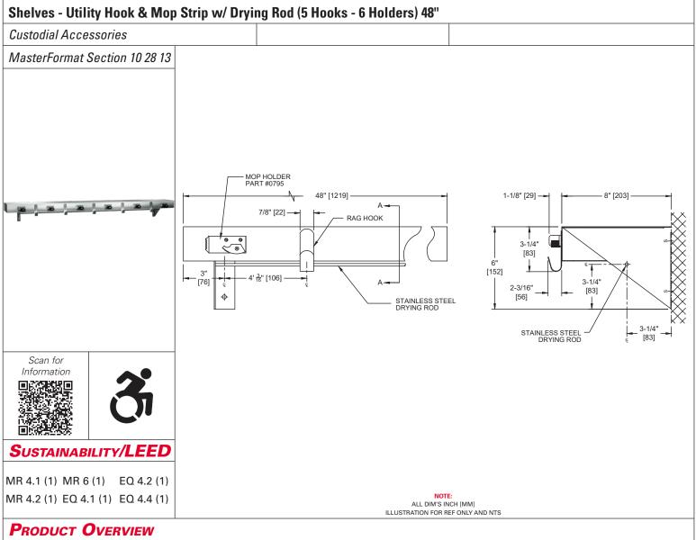
Shelf fabricated of 18 gauge type 304 satin finish stainless steel, this shelf is 8" [203] deep with 3/4" [19] return for rigidity, mounting brackets shall be 16 gauge same material. Mop holders are riveted to strip, and rubber cam is ribbed for grasping. Rod and hooks for wet rags are included. 6 mop holders/5 rag hooks, 48" [1219]. Pivoting spring loaded holders have serrated rubber cams for grasping.
