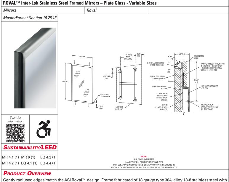
Gently radiused edges match the ASI Roval<sup>™</sup> design. Frame fabricated of 18 gauge type 304, alloy 18-8 stainless steel with satin finish and polished seamless mitered corners. 0.25" [6.4] thick plate glass mirror. See Price List for all sizes available. Variable sizes available.
