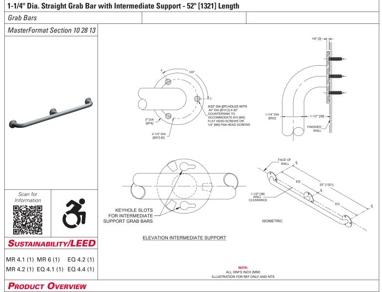
Features include flange of 3" diameter [Ø76], 1/8" [3] thick type 304 stainless steel with a satin finish; exposed mounting screw holes are drilled and countersunk. 1-1/4" outside diameter [Ø32] bar with smooth surface.
