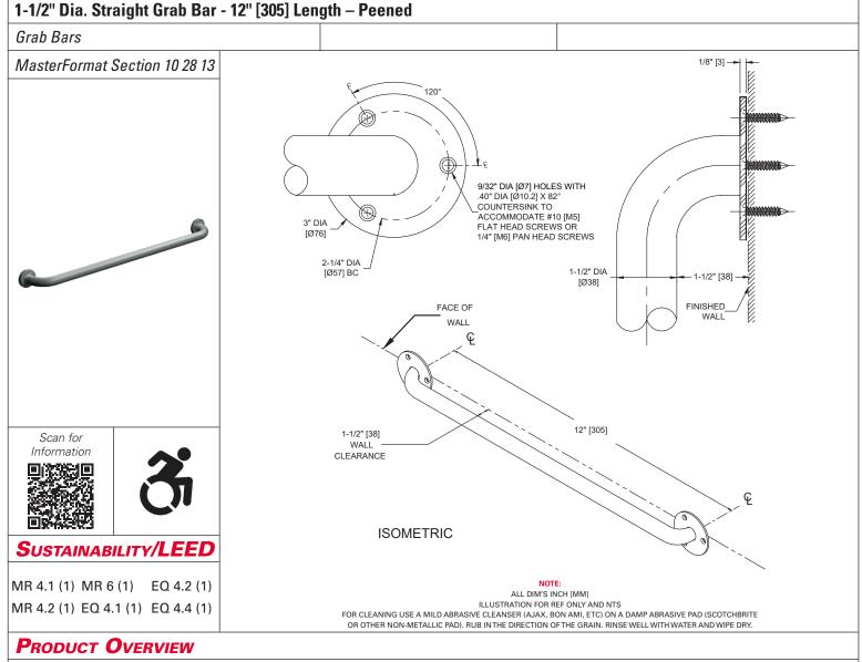
Features include flange of 3" diameter [Ø76], 1/8" [3] thick type 304 stainless steel with a satin finish; exposed mounting screw holes are drilled and countersunk. 1-1/2" O.D [Ø38] exposed flange horizontal grab bar with a peened surface.
