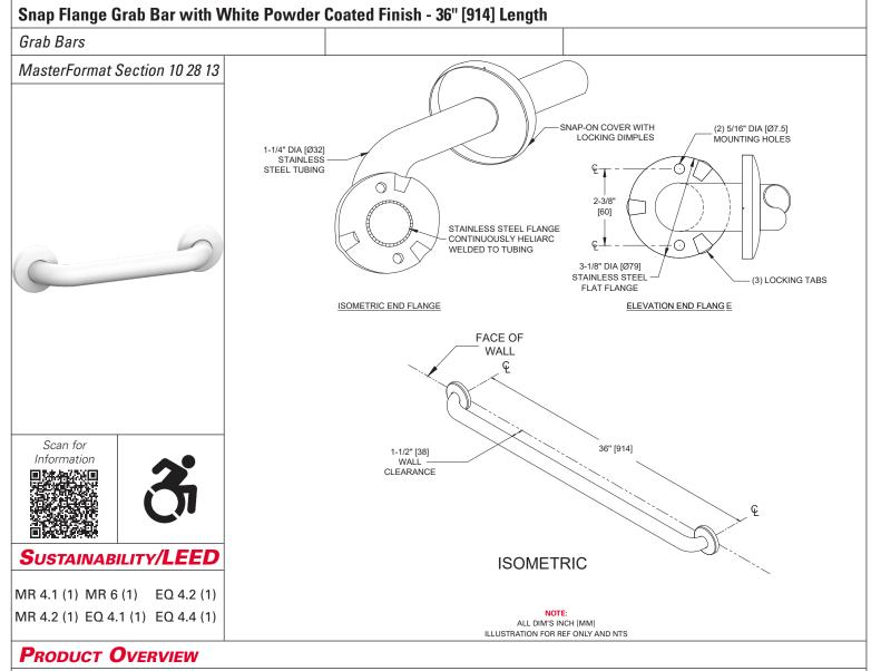
Features include cover that snaps over mounting flange dimples to conceal screws and concealed mounting flange of 3-1/8" O.D. [Ø79] with 2 screw holes and 3 locking dimples; 1/8" [3] thick, type 304 stainless steel. Cover is type 304 stainless steel with a satin finish and 22 gauge, 3-3/16" [81] diameter.
