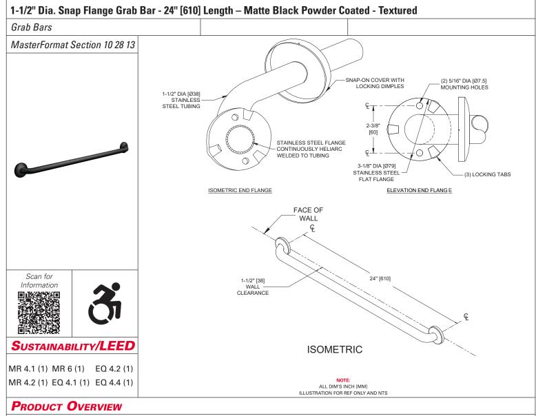
Features include cover that snaps over mounting flange dimples to conceal screws and concealed mounting flange of 3-1/8" [79] O.D. with 2 screw holes and 3 locking dimples; 1/8" [3] thick, type 304 stainless steel. Cover is Matte Black Powder Coated type 304 stainless steel with a 22 gauge, 3-3/16" [81] diameter. 1-1/2" O.D [Ø38] horizontal grab bar with texture for easier grabbing.
