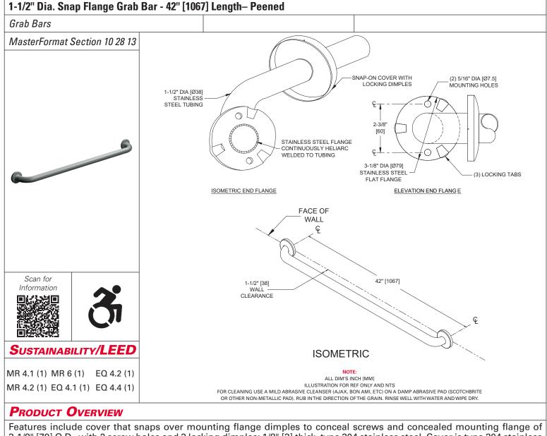
Features include cover that snaps over mounting flange dimples to conceal screws and concealed mounting flange of 3-1/8" [79] O.D. with 2 screw holes and 3 locking dimples; 1/8" [3] thick, type 304 stainless steel. Cover is type 304 stainless steel with a satin finish and 22 gauge, 3-3/16" [81] diameter. 1-1/2" O.D [Ø38] horizontal grab bar with peened surface for easier grabbing.
