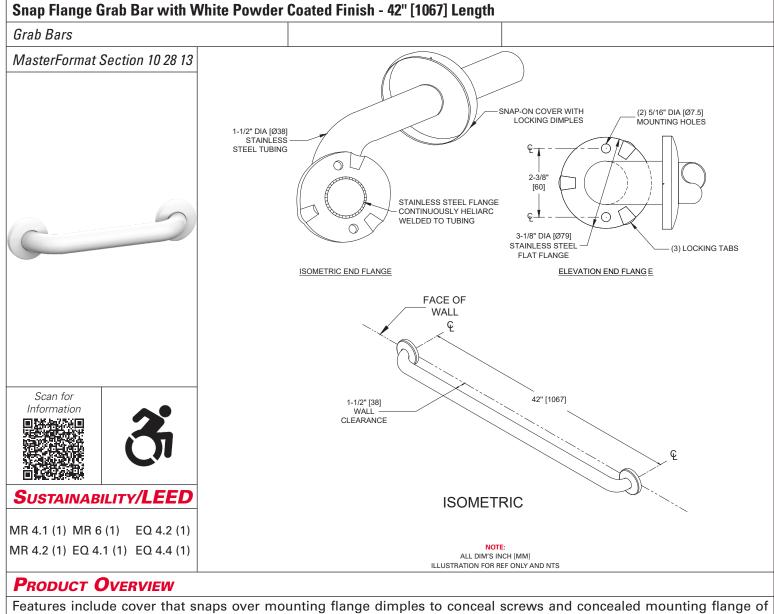
3-1/8" [79] O.D. with 2 screw holes and 3 locking dimples; 1/8" [3] thick, type 304 stainless steel. Cover is type 304 stainless steel with a White Powder Coated Finish and 22 gauge, 3-3/16" [81] diameter. 1-1/2" O.D [Ø38] horizontal grab bar. - white powder coat finish.
