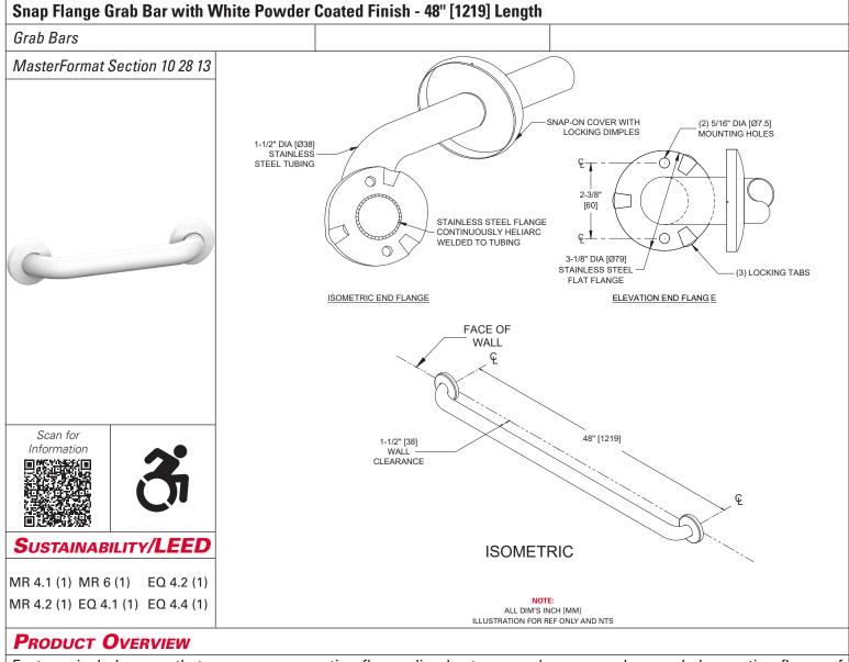
Features include cover that snaps over mounting flange dimples to conceal screws and concealed mounting flange of 3-1/8" [79] O.D. with 2 screw holes and 3 locking dimples; 1/8" [3] thick, type 304 stainless steel. Cover is type 304 stainless steel with a White Powder Coated Finish and 22 gauge, 3-3/16" [81] diameter. 1-1/2" O.D [Ø38] horizontal grab bar. - white powder coat finish.
