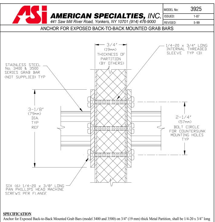
Anchor for Exposed Back-to-Back Mounted Grab Bars (model 3400 and 3500) on 3/4" (19 mm) thick Metal Partition, shall be 1/4-20 x 3/4" long female threaded posts with 1/4-20 x 3/8" long phillips pan head machine screws. Anchor kit shall contain (3) female posts and (6) machine screws. Specify one (1) kit **per flange.**
