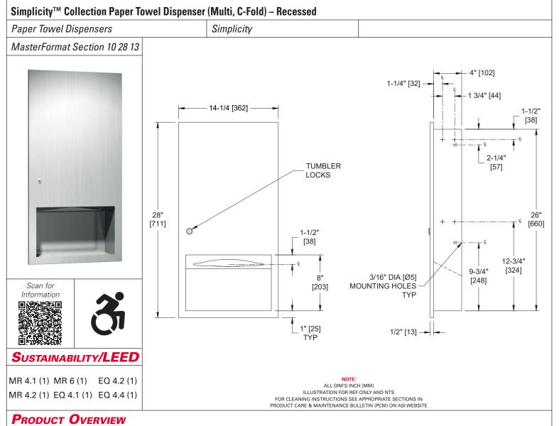
Holds and dispenses 600 C-fold or 800 multi-fold paper towels. Door held closed with a tumbler lock. All exposed surfaces have a satin finish. Towels are self-feeding until supply is depleted. Unit may be reloaded with a partial load in-place and will continue to feed properly. Locking door prevents unauthorized access or removal.
