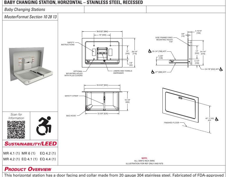
fungus and bacteria-resistant plastic. Unit complies with 2010 ADA Accessibility Standards, ASTM F-2285 & F-2388, G-21, G-22, ANSI Z535, ANSI 117.1, EN 12221-1, and EN 12221-2 (Including A1:2013). Tested during development to sustain 250 Ibs (113 kg) static load with minimal deflection. Recessed Mounting.
